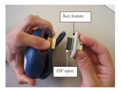
6. Align the key feature on the bulkhead and the BISx unit. Attach the flex cable from the BISx to the ZIF connector on the replacement bulkhead.
