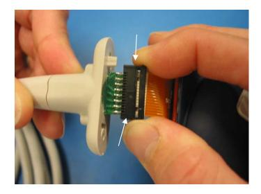
3. Open the ZIF connector by pulling away from the bulkhead.
