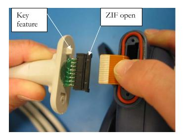
6. Align the key feature on the bulkhead and the BISx unit. Attach the flex cable from the BISx to the ZIF connector on the replacement cable.
