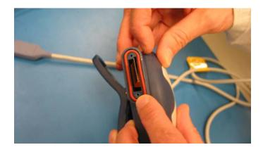
5. Set the new gasket in the groove of the BISx housing.
