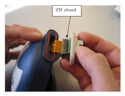
7. Ensure that the flex cable is fully inserted into the ZIF and close the ZIF connector by pushing toward the bulkhead. Carefully feed the flex cable into the housing and seat the bulkhead to the BISx housing.
