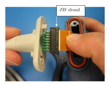
7. Ensure that the flex cable is fully inserted into the ZIF and close the ZIF connector by pushing toward the bulkhead. Carefully feed the flex cable into the housing and seat the cable bulkhead to the BISx housing.
